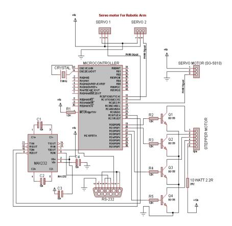
Figure 9: Electric Schematic Diagram of the Control Board
