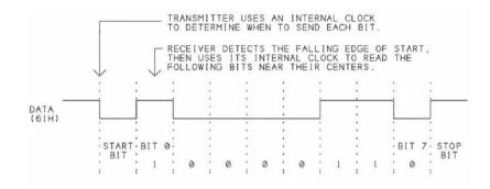
Figure 10: Basic Asynchronous Data Transmission System [9]
