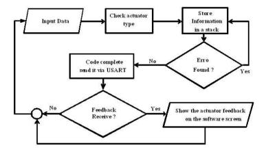
Figure 7: Flow Chart of the Software Algorithm
