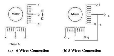
Figure 2: Example of Various Stepper Motor Wire Configuration
