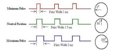
Figure 5: PWM Signal for Servo Motor Position Control
