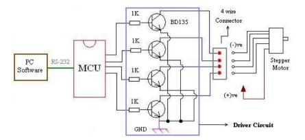
Figure 4: Stepper Motor Driver Circuit for 5 Wires
